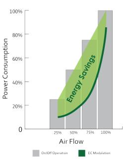
EC fans have **high efficiency over a wide operating point** because the **integrated components are optimised for each other**. AC fans are not able to replicate this.
