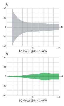
0 – 100% continuous speed control (Right): In AC motors, there are limited speed settings. This results in energy wastage. In contrast, EC motors can regulate energy use based on the conditions of the environment, resulting in high energy efficiency.
